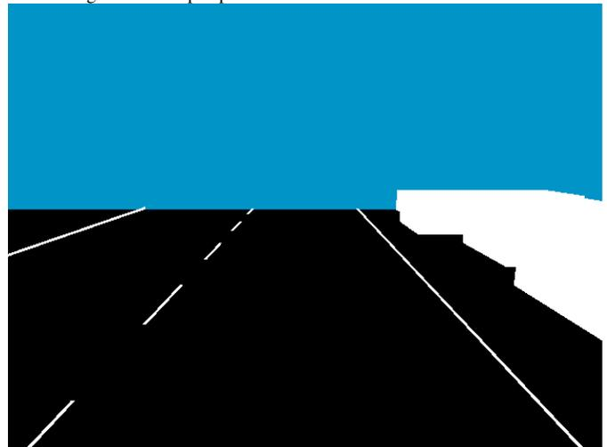
of the simulated environment from the car's perspective [Fig. 7] as well as bird's eye view of the map [Fig. 8]. We can also accelerate and steer the vehicle around. The scenario editor lets us modify or create new tracks. With these tools, it is possible to build and test a comprehensive lane detection
