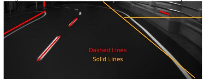
1) *Classify Lines*: The rectangles are approximated into lines according to their vertices and are then classified into solid or dashed lines. The classification is done by comparing the ratio between width and height of the rectangles or their
