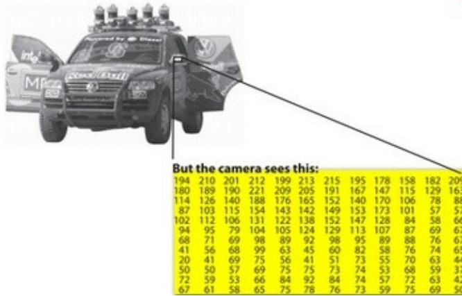
as a matrix of colours [Fig. 1, 2]. Each matrix element holding an array of integers describing the colour using a combination of colour channels, e.g. red, green and blue; cyan, magenta, yellow and black; shades of grey; black and white. An element, unit or item of an image matrix is often referred to as *pixel*.
